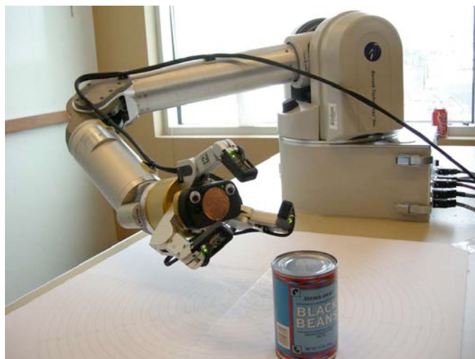
Fig. 1. Photograph of Electric Field Pretouch manipulation system. The system includes a WAM arm and Barrett Hand. Each fingertip contains one of our custom Electric Field Sensing boards and 4 sensing electrodes. Another EF sensing board with one transmit electrode is built into the palm. The palm board also serves as a hub for aggregating sensor data from the fingertips. The palm also contains a camera, which was not used in the experiments reported in this paper. The googly eyes also were not used. A polar coordinate system used for mapping the region of where the grasping procedure succeeds is visible beneath an example object (a can).
