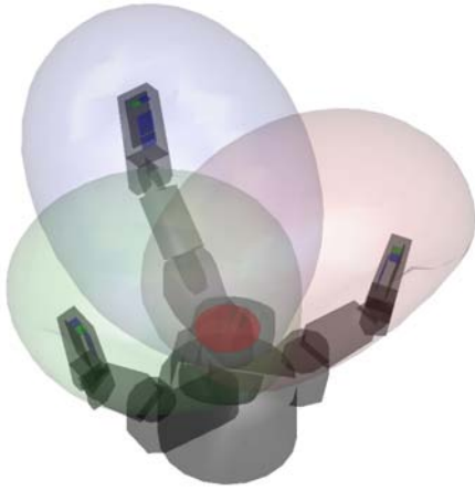
Fig. 6. Iso-signal surfaces for the hand's long-range measurements.
