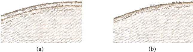
Fig. 2: Zoom into the edge of the table from Fig. 1: (a) after SIFT RANSAC alignment; (b) after additional ICP alignment.
