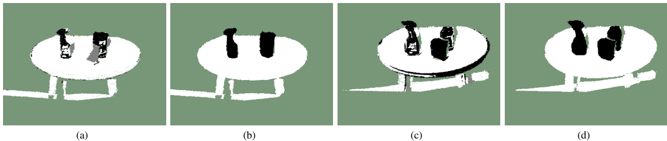
Fig. 5: (a) surfel-wise differencing and (b) regularization results for the first scene of Fig. 1; (c), (d) similarly for the second scene.
